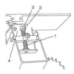
You can place a small amount of dry lubricant on bevel angle adjustment rod also. This rod (1) must be kept clean and free of sawdust, gum, pitch, and other contaminants for smooth operation.
